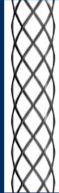
As the Width : Height ratio gets closer, radial strength is less and the stent overall is longer
